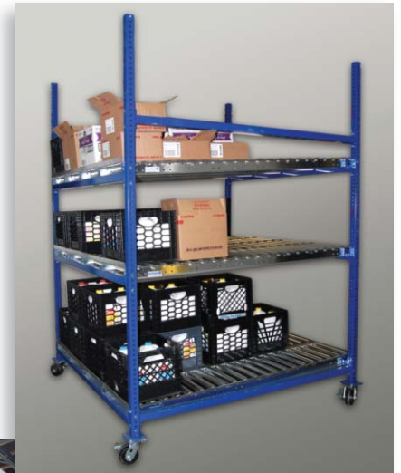
Right: UNEX's custom engineered flow rack for Capital Candy's dairy line.
