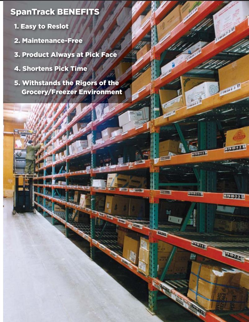
Worker loads product from back of rack. SpanTrack consistently flows product to “last in” position for strict inventory rotation.
