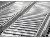
**Guard Rail – Lane** Guard rails that bolt onto the side of the track. 4 spacer widths available with in- or outflange configuration.
